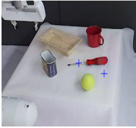
(a) Grasp area demonstrations via interactive segmentation. The selected region on the screwdriver handle is shown in red.
