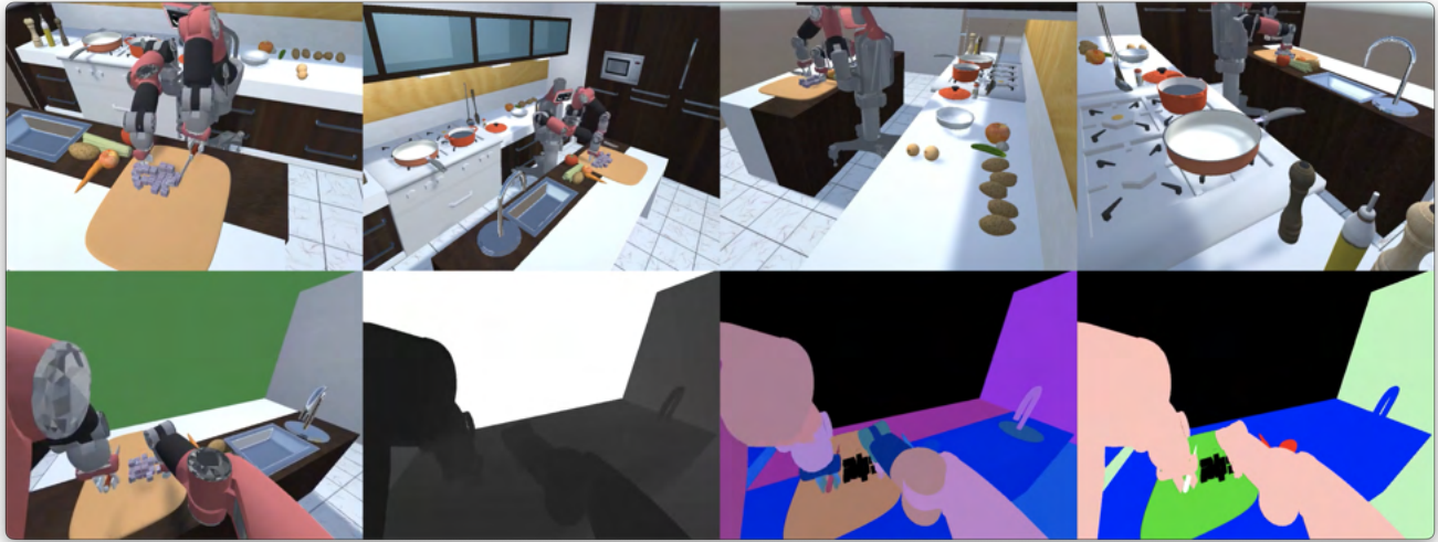
Figure 2: Our Simulator that shows Baxter cutting onions into pieces. The simulator includes multi-view perspectives of the scene and the robot from fixed and moving cameras. The top row shows human-first-person view, the ceiling top left, the counter bottom right, and counter bottom left cameras in the kitchen. The bottom row shows robot’s egocentric view in RGB, depth, unique object segmentation, and category based semantic segmentation. These perspective are useful for robot to learn to complete the tasks based on human speech-gesture commands and it’s own observation of the world and object states.
